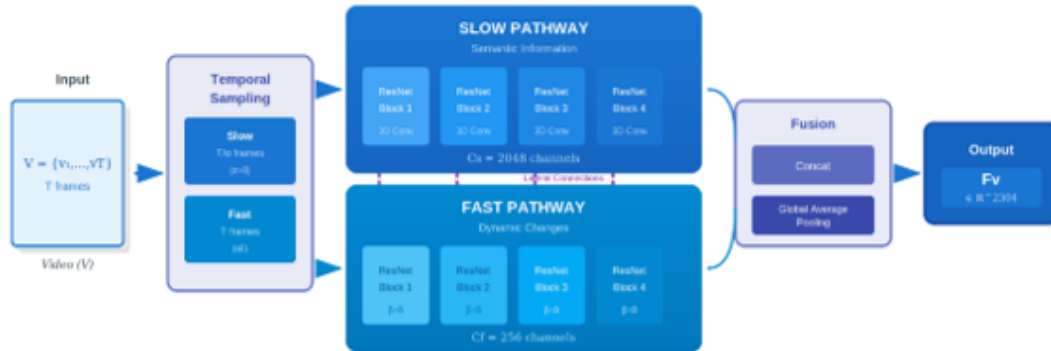
Figure 2 Visual Feature Extraction Module (VFM) architecture
